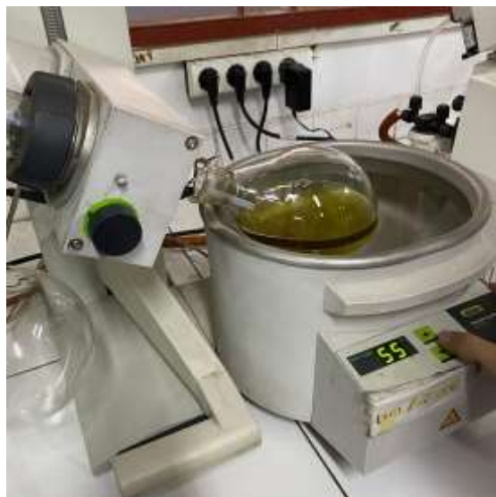
Picture 2. Rotary Vacuum Evaporator Apparatus
